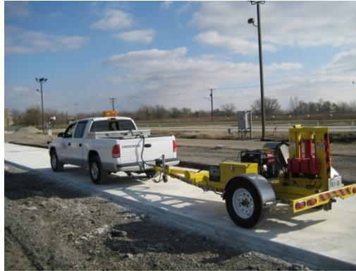
Figure 19. FWD used for center slab deflections and joint load transfer efficiency.
